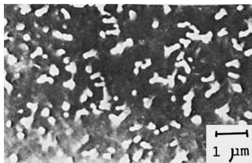
Fig. 6. SEM micrographs of PE75EPDM25 blend; higher magnification ( \times 15,000 ).
